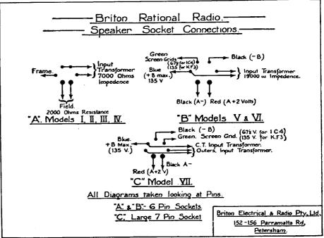
Above are shown the loudspeaker and loudspeaker-battery plug connections used with "Briton" models 1 to 7A, inclusive. Since the above block was made, Briton's address has been changed to 369 Kent Street, Sydney.
