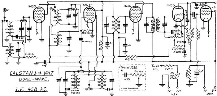
The Calstan "1.4 volt" dual-wave receiver is primarily designed for portable service and is made up on a compact chassis with the speaker built on to the frame. The speaker is a Rola six-inch dust-proof unit with an 11 oz, magnet and a transformer input impedance of 8,000 ohms. Power supply for this receiver is obtained from a 1.5-volt "A" battery and two series-connected 45-
