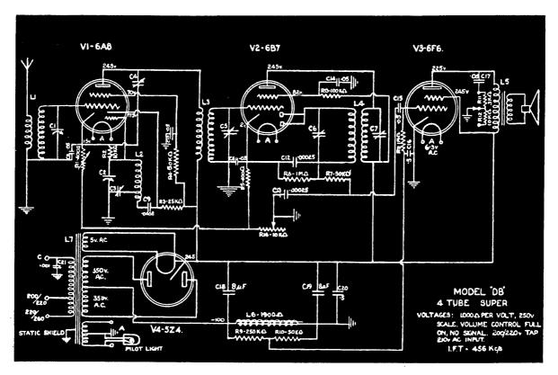
Astor model "55." chassis type "DB." is a four-valve receiver designed for broadcast coverage and operation from 200-260 volts A.C. mains. This receiver is of the console type and is fitted with three controls—volume, tuning, tone (3 positions)—and an 8 inch, 1,900 ohms field. loudspeaker
