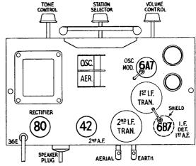
6A7 (ON): Cathode, 2 v.; screen, 90 v.; plate, 250 v.; oscillator plate, 130 v.
