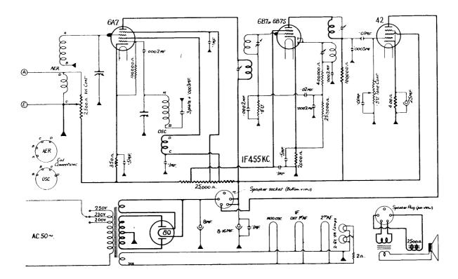
The controls fitted to this receiver number three in all, and are for one, tuning and volume. Their disposition is shown on the toptone, tuning and volume. Their disposition is shown on the top-chassis layout drawing. Reference to the circuit diagram will show that the tone control also serves as grid-resistor for the output valve, and also that the volume control is of the "R.F." type which controls the aerial input simultaneously with the bias applied to the frequency
