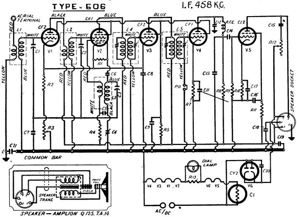
Lekmek model "606" is a six-valve, broadcast receiver designed for operation from 200-260 volts A.C. or D.C. mains. This receiver is of the console type and is fitted with three controls — volume. tuning, and tone (continuous). The loudspeaker is an 8-inch unit with a field coil resistance of 1,250 ohms.
